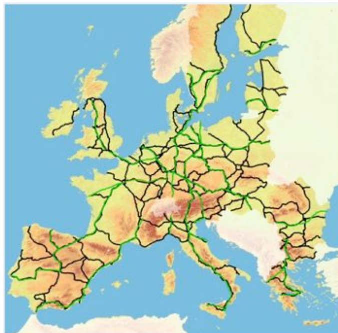
Overlap between the TEN-T core network (in black) and SuperGreen corridors (in green). Land-based and inland waterway corridors only.
